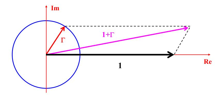
We can use a geometric construction to visualize the behavior of the voltage standing wave pattern
