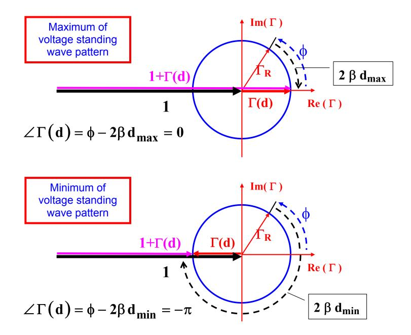
The voltage standing wave ratio (VSWR) is an indicator of load matching which is widely used in engineering applications
