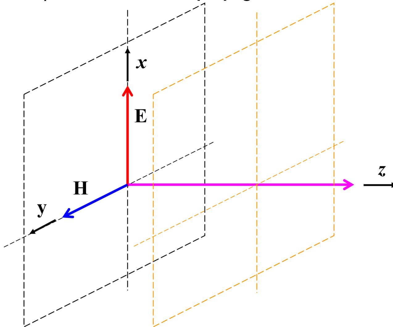
**Electromagnetic power** flows with the wave along the direction of propagation and it is also constant on the phase-planes. The **power density** is described by the time-dependent **Poynting vector**
