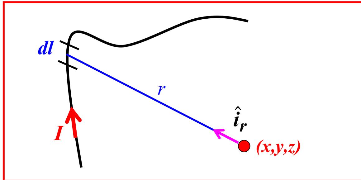
The **magnetic field** can also be determined by **direct integration** of the curl equation over a surface
