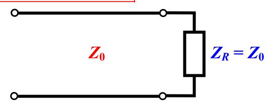
The reflection coefficient for a matched load is
