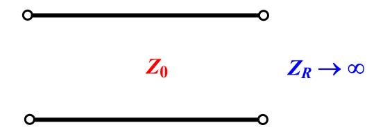
The load boundary condition due to the open circuit is I(0) = 0
