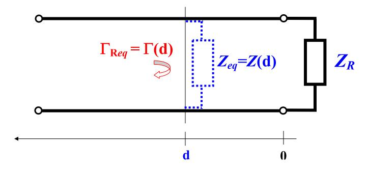
If you imagine to cut the line at location d, the input impedance of the portion of line terminated by the load is the same as the line impedance at that location "before the cut". The behavior of the line on the left of location d is the same if an equivalent impedance with value Z(d) replaces the cut out portion. The reflection coefficient of the new load is equal to  $\Gamma(d)$
