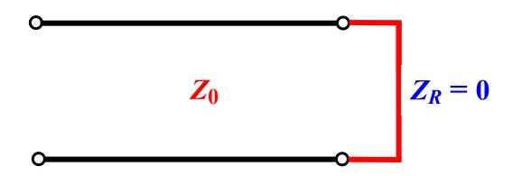
The load boundary condition due to the short circuit is V(0) = 0
