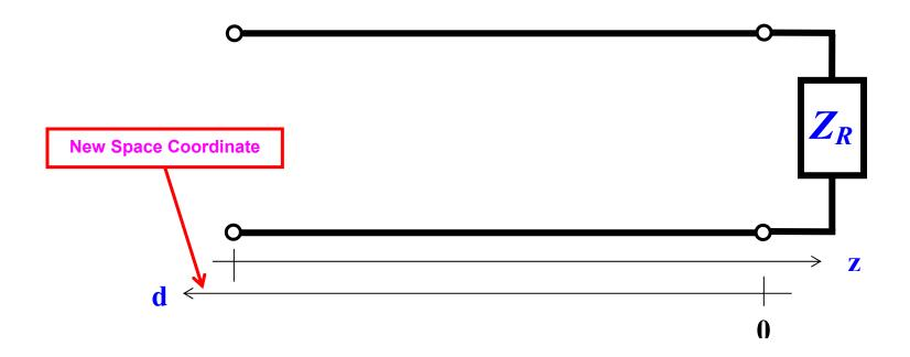
We will also change the positive direction of the space coordinate, so that it increases when moving from load to generator along the transmission line.
