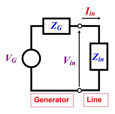
$$V_{in} = V_G \frac{Z_{in}}{Z_G + Z_{in}}$$
