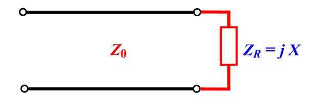
The reflection coefficient for a purely reactive load is
