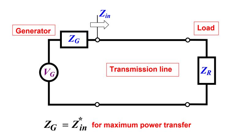
The characteristic impedance of the loss-less line is real and we can express the power flow, anywhere on the line, as
